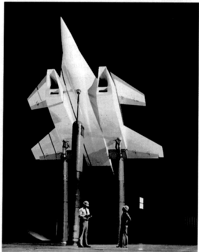
FIGURE 3.38 Aircraft Model Being Prepared for Wind Tunnel Studies
